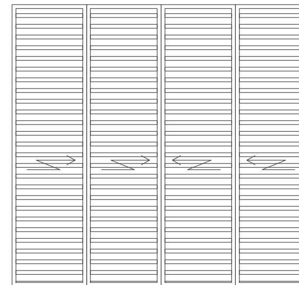
TYPICAL ELEVATION - BALCONY SCREEN
